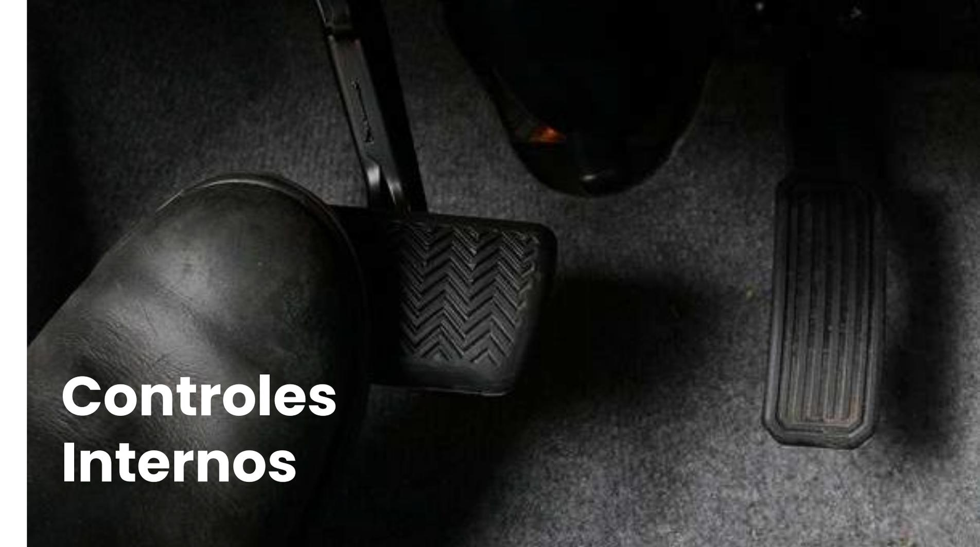
A close-up, low-angle shot of the interior of a car, focusing on the three pedals: the clutch on the left, the brake in the center, and the accelerator on the right. The pedals are black with textured surfaces. The floor is covered in a dark, textured carpet. The lighting is dramatic, with strong highlights on the pedals and deep shadows in the surrounding areas.
